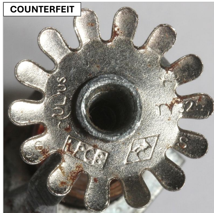
Figure 9. Deflector markings on the counterfeit TY325
