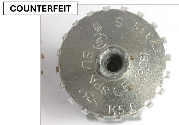
Figure 7. Markings on the deflector of the counterfeit TY3151
