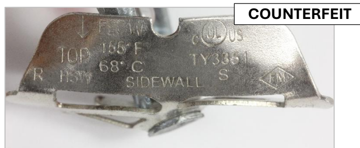
Figure 2. Photograph of the deflector markings on the counterfeit TY3351
